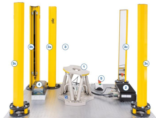
Fig. 5 The hexapod is surrounded by the safety light barrier on four sides. 1: Hexapod. 2: C-887 hexapod controller. 3: Safety light curtain. 3a: Emitter. 3b: Receiver. 3c: Mirror. 4: Safety relay, relays, power supply. 5: Emergency-stop switch, reset button
