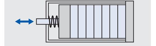
The piezo ceramic stack is mechanically preloaded against the housing by means of a spring. This prevents pull forces, such as the ones caused by the inert mass of the load in dynamic operation
