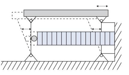
Simple lever amplification. The point contact decouples shear forces and thus tensile stress on the piezo ceramic
